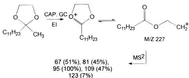
**Scheme 1.** Independent method for generation of a carbonium ion of the class  $[R-COX-(CH_2)_nCH_2]^+$  by capillary GC/electron ionization MS/MS, where  $X=O$  and  $n=1$ , with resultant product ions and relative abundances listed.
