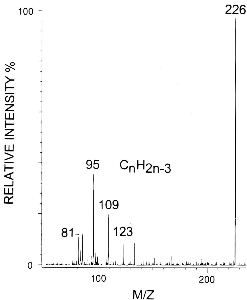
Figure 4. Electrospray positive ion MS<sup>3</sup> analysis ( $345^+ \rightarrow 226^+$ -product ions) of the infused shampoo extract.
