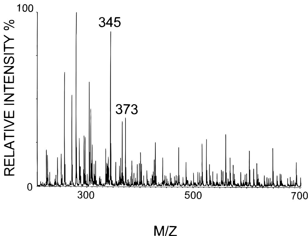
**Figure 1.** Electrospray positive ion mass spectrum of the infused ( $5 \mu\text{l min}^{-1}$ ) shampoo extract, obtained using a triple-sector-quadrupole mass spectrometer.
