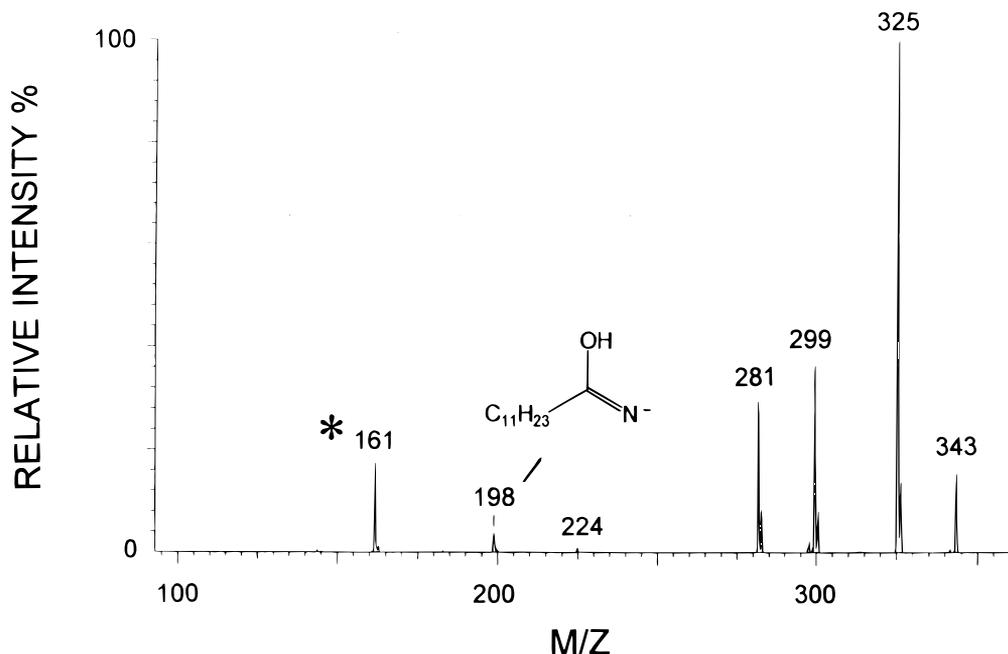
**Figure 6.** Electrospray negative ion product ion mass spectrum of  $m/z$  343 from the infused shampoo extract ( $5 \mu\text{l min}^{-1}$ ). The peak marked with an asterisk contained the structural elements not found in positive ion analysis.
