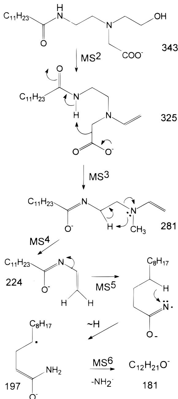
**Scheme 5.** One negative ion  $\text{MS}^n$  pathway of decomposition observed for electro sprayed lauryl amphoacetate, with  $m/z$  values and suggested structures of ions.
