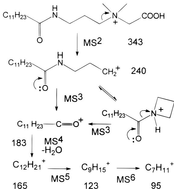
**Scheme 2.** One positive ion  $MS^6$  pathway of decomposition observed for electrosprayed laurylbetaine, with  $m/z$  values and suggested structures of the ions.
