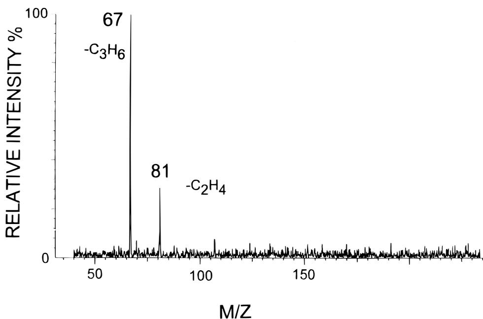
Figure 5. Electrospray positive ion MS<sup>4</sup> analysis ( $345^+ \rightarrow 226^+ \rightarrow 109^+$ -product ions) of the infused shampoo extract.
