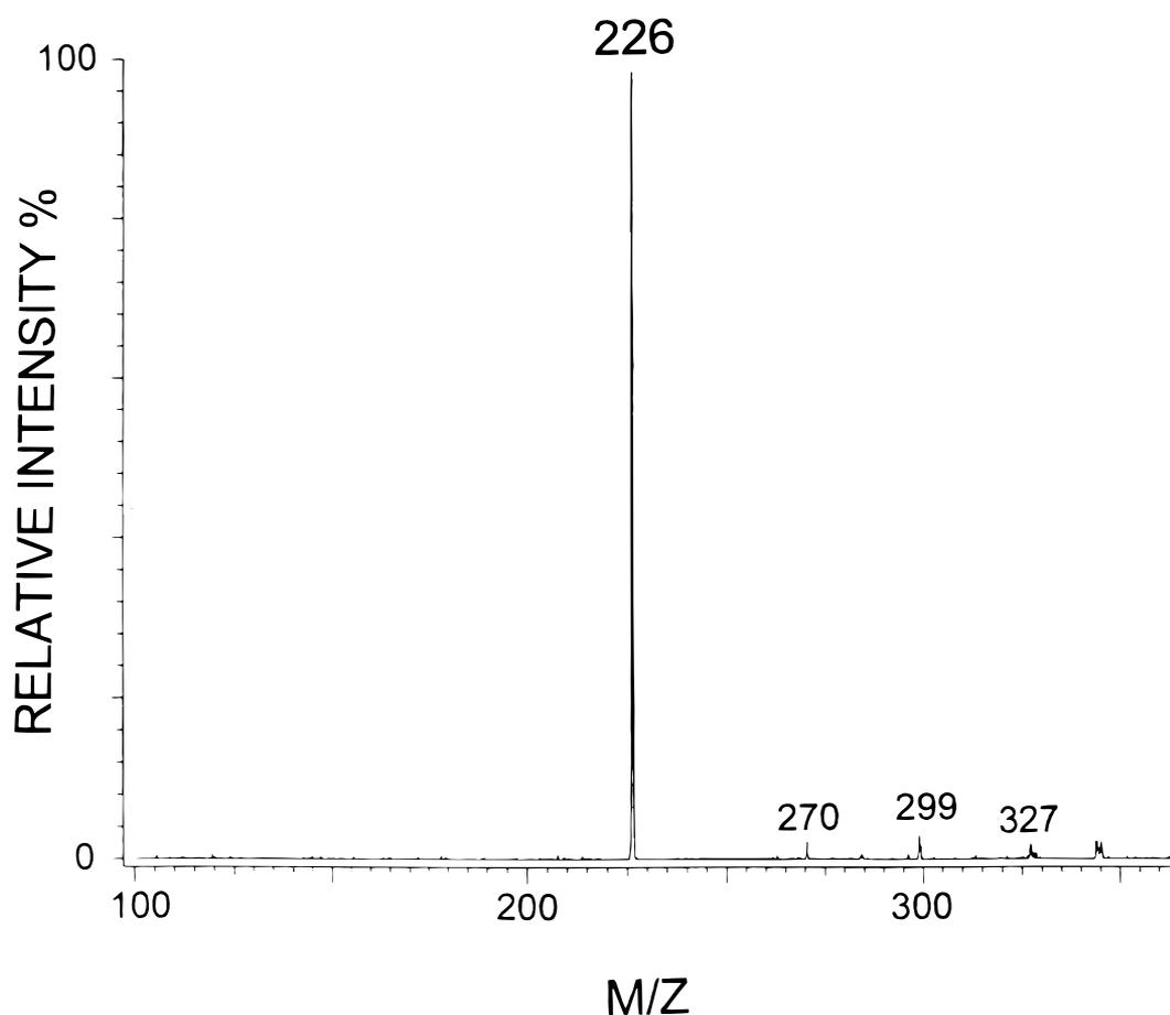
**Figure 2.** Electrospray positive ion product ion spectrum of  $m/z$  345, obtained on the sample whose spectrum is shown in Fig. 1. The collision energy ( $\text{Ar}^0$ ) was 25 eV in the laboratory frame of reference.
