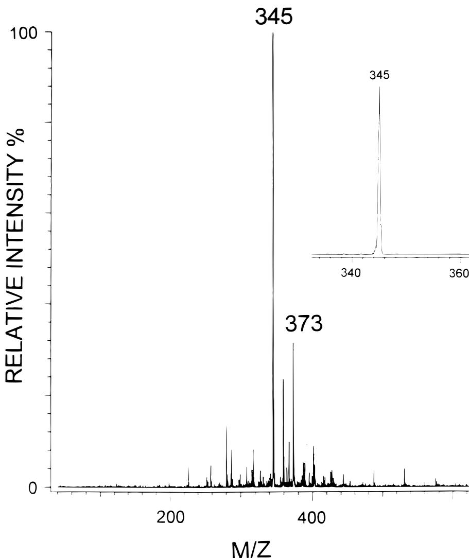
**Figure 3.** Electrospray positive ion mass spectrum of the infused shampoo extract ( $5 \mu\text{l min}^{-1}$ ). The spectrum was obtained using the quadrupole ion trap with ion injection. The inset shows the result of application of an isolation waveform for  $m/z$  345.
