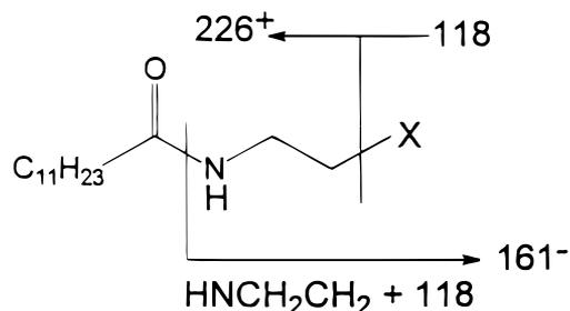
**Scheme 3.** Summary of possible structural content of  $m/z$  161<sup>-</sup> and  $m/z$  226<sup>+</sup>.
